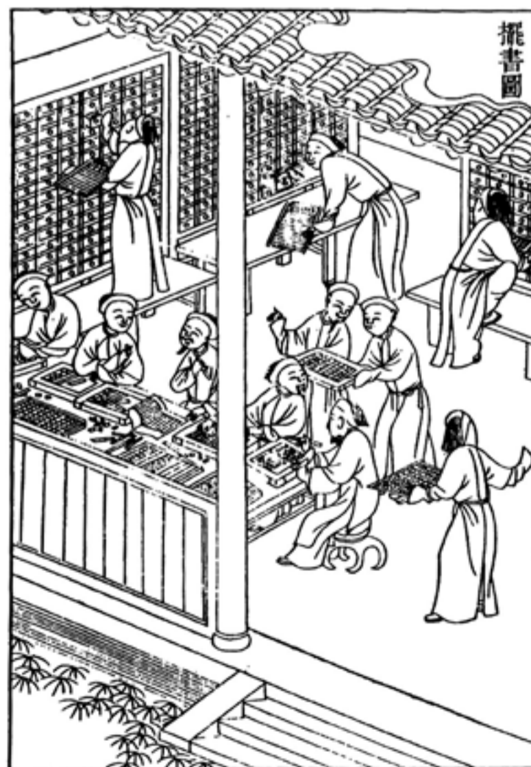
Setting movable type in the Qianlong Imperial Printing Office. Qinding Wuying dian juzhen ban chengshi (Beijing, 1776). Elman, Benjamin A. 2005. On their Own Terms: Science in China, 1550-1900. p. 18
