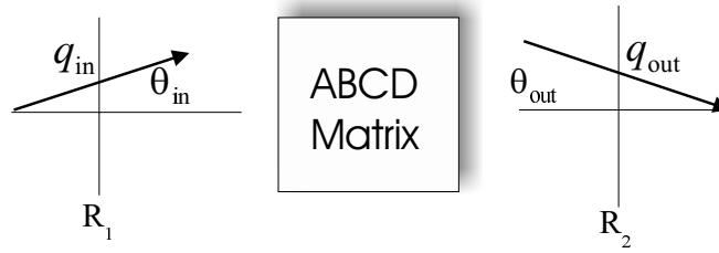
Figure 1.2: The input canonical variables (q_{\text{in}}, \theta_{\text{in}}) , specifying a ray on a reference plane R_1 , are mapped by the ABCD matrix into the output canonical variables (q_{\text{out}}, \theta_{\text{out}}) of a ray on a reference plane R_2 .
