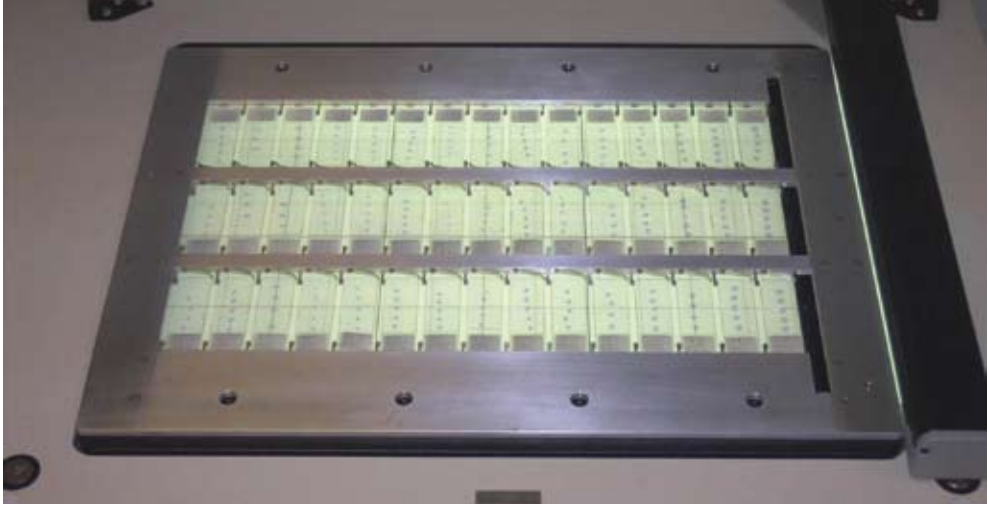
Fig. 1 A3-size mold to hold 15 \times 3 = 45 slides on the AGFA XY15 scanner. Each slide may contain several tissue sections.
