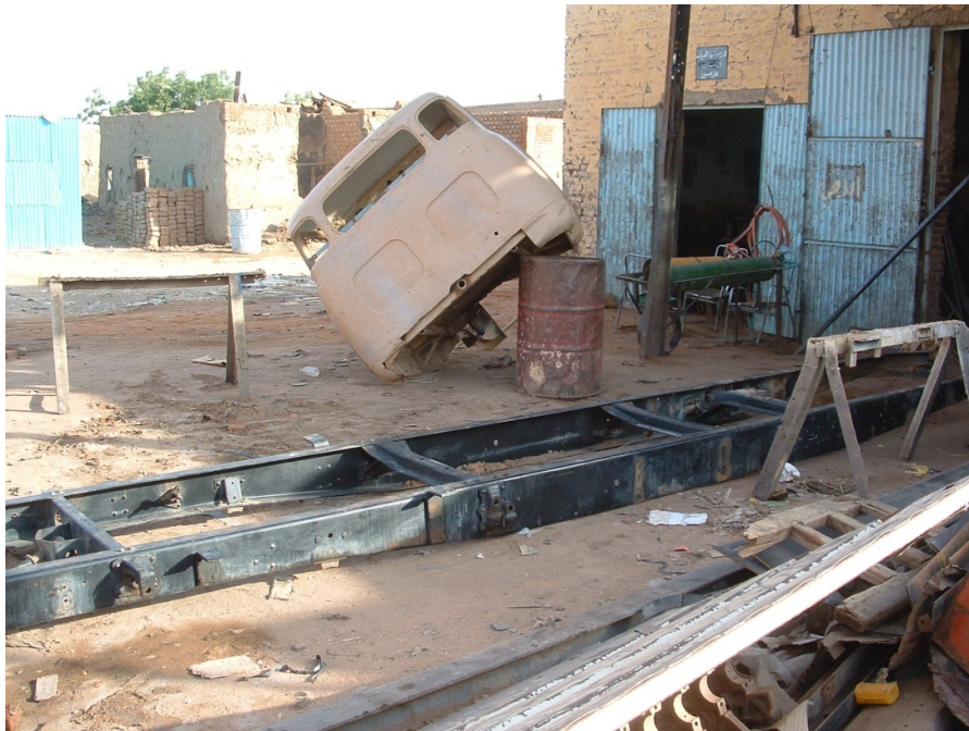
Photo 6.4 Bedford TJ dismantled Source: K. Beck
