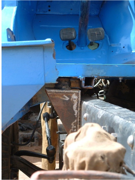
Photo 6.7 Reinforcing the cabin Source: K. Beck
