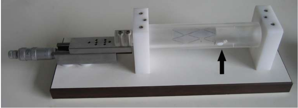
Figure 1. Model used in the experiments. The micromanipulator can displace the stent in a highly controlled manner along the axis of the aorta. Markers are placed on the stent and inside the aorta for RSA analysis. Renal arteries (arrow) are mimicked by polytetrafluoroethylene inlays in the wall of the aorta for CT analysis.
