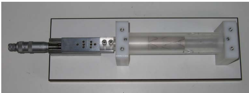
Figure 5. Static model of an aorta (tube) with stentgraft (visible inside tube). Micromanipulator is on the left side.
