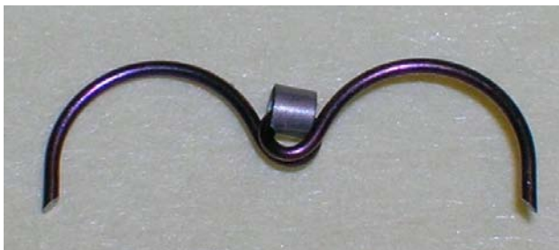
Figure 5. Platinum ring attached to the nitinol endovascular clip for enhanced radiopacity.
