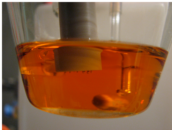
Fig. 3.9. Dihydrogen bubbles formed on the surface of the glassy carbon working electrode during the electrocatalysis of 0.5 mM [Ni(pbss)Fe(C 5 H 5 )(CO)]PF 6 in the presence of acetic acid. Object at the bottom of the cell is a stir-bar; the Pt wire counter electrode and the Ag/AgCl reference electrode are behind the working electrode.
