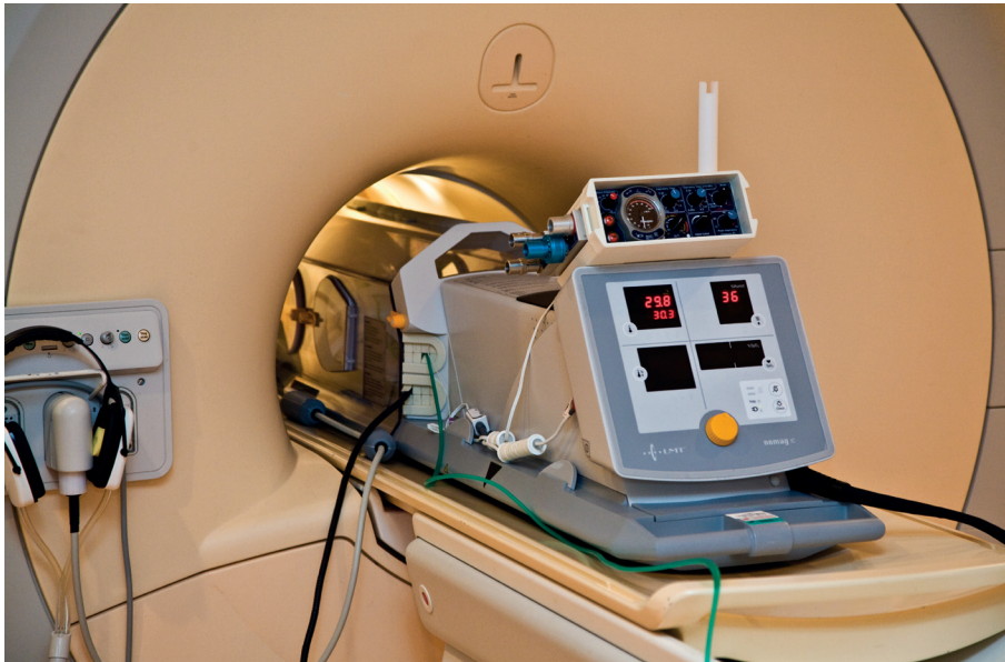
Figure 6. MRI incubator, removed from the trolley and installed on the MR table. Also showing the MR-compatible ventilator.
