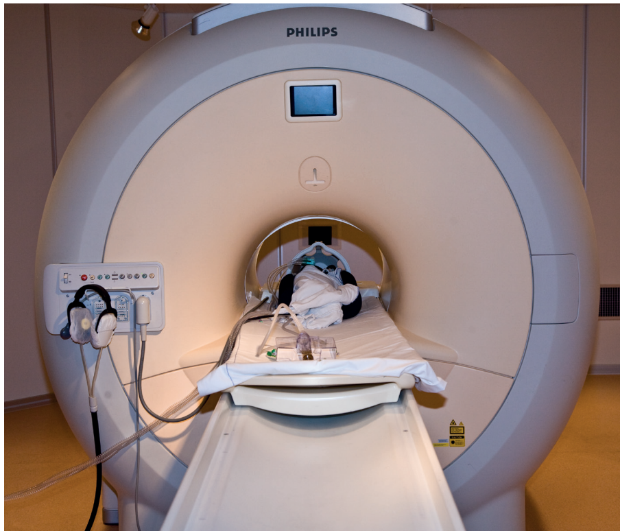
Figure 8. The ventilated neonate is installed in the scanner. Note the extended ventilation hoses and intravenous lines guided to the hole in the wall.
