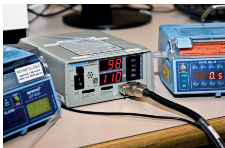
Figure 3. MR-compatible pulse oximeter with fibre-optic lead, positioned in the control room of the 3 Tesla MR unit. Also showing standard (not MR-compatible) intravenous pumps.
