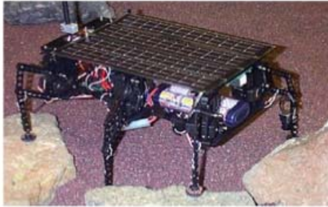
Figure 10. A small surface robot in the 5-kg class. Image Credit: Jet Propulsion Laboratory
