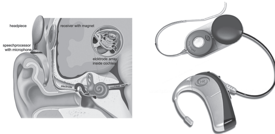
Figure 1: a) Schematic drawing of a cochlear implant. A cochlear implant consists of an externally worn speech processor and a microphone. The speech processor filters, analyzes and converts the auditory signals captured by the microphone to a digital code. A head piece containing a transmitting coil sends the signal from the speech processor to a subcutaneous implanted receiver to which it is magnetically attached. The receiver contains electronics to decode the signals and generate electrical stimuli. An electrode array is connected to this receiver and inserted into the scala tympani of the cochlea. The electrical stimuli sent to the electrode array will bypass the damaged parts of the cochlea and directly stimulate the auditory nerve. In multichannel arrays the electrode array contains several electrode contacts to ensure well directed stimulation of the tonotopically organized cochlea. b) Cochlear implant (Advanced Bionics HiRes 90k and Auria speech processor). The external and internal components of the implant are shown. The behind the ear part contains the speech processor and a built-in microphone. Alternatively a body worn processor can be used. Implants of other manufacturers have a slightly different appearance, but contain the same components.
