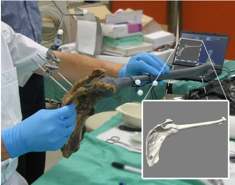
Figure 4.5: Real-time motion tracking. Marker trees are attached to each bone, and these are tracked by the infra-red guidance system. The intra-operative tracking system on the laptop shows the real-time position and orientation of the tracked bones.
