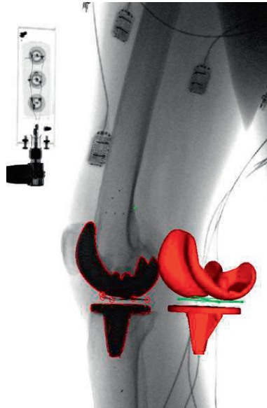
Figure 4.2: An analyzed fluoroscopic image showing the reversed engineered models of the femoral and tibial component and the marker model of the insert and their 2D projections. In addition, the custom made box with X-ray sensitive photocells (upper left corner) used for temporal synchronisation, and three EMG electrodes placed on the upper leg are visible.
