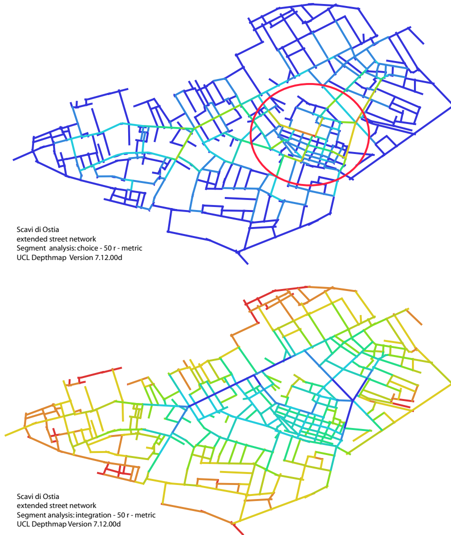
Fig. 7.13 – Segment analysis graphs for 50 m radius: choice and integration
