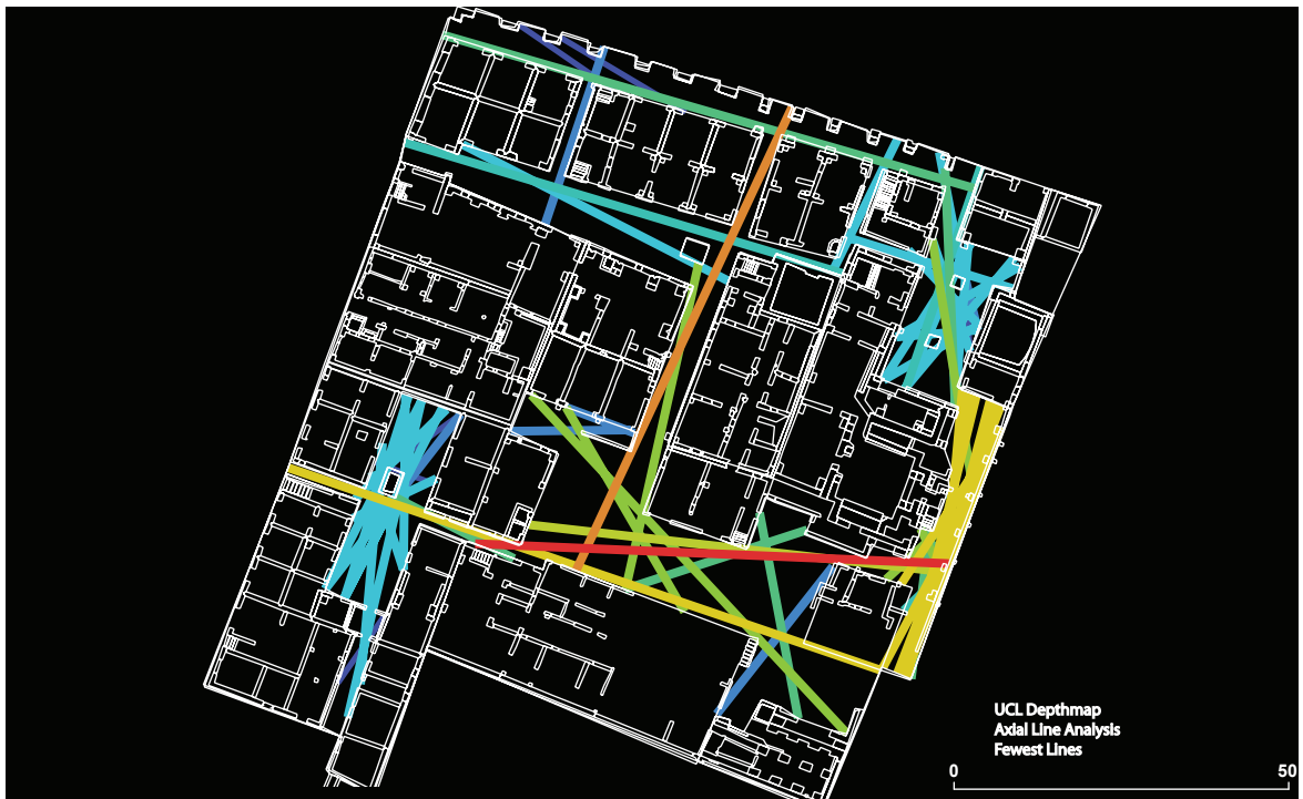
Fig. 6.21 – The Insula’s potential route matrix based on the longest and fewest lines, including the movement spaces of the Terme del Faro
