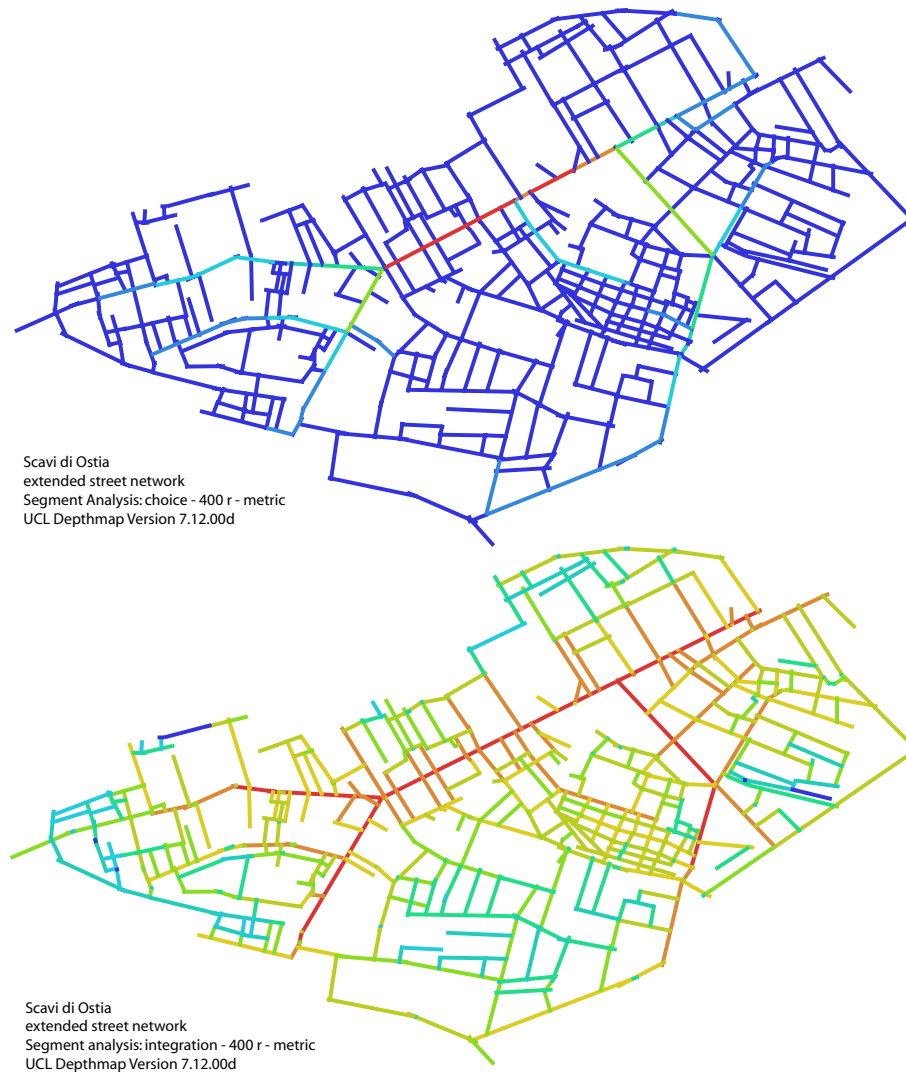
Fig. 7.12 – Segment analysis graphs produced for 400 m radius: choice and integration
