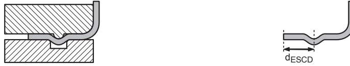
Figure 9.1: U-Profile experiment; Left: Definition of the binder zone; Right: Definition of the d_{ESCD} .
