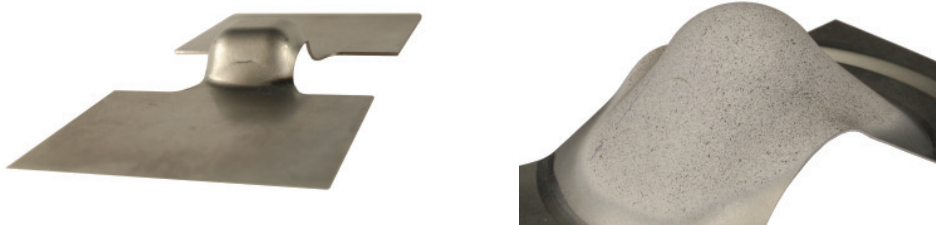
Figure A.2: YLIT-Experiments; Left: Shape of the specimen of the YLIT-3-BMW after forming; Right: Shape of the specimen of the YLIT-4-BMW after forming.
