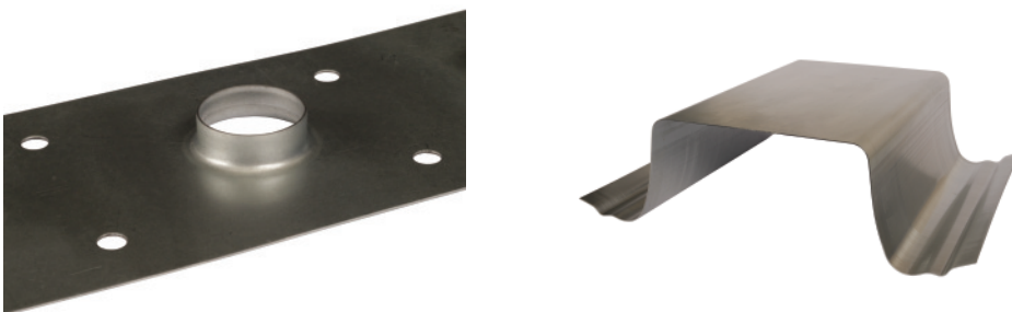
Figure A.4: Left: Hole extrusion experiment; The shape of the specimen after the forming operation; Right: U-Profile experiment; The shape of the specimen after the forming operation.
