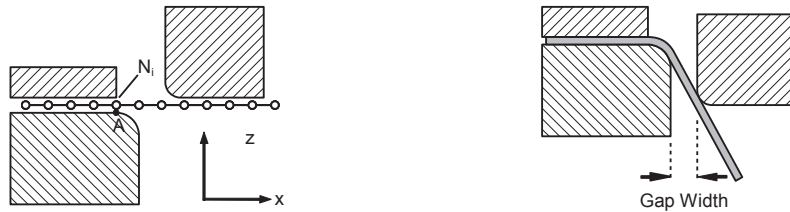
Figure 8.42: Bending experiment; Left: For the generation of the mesh of the specimen, the depicted nodes are assumed to be extruded in y -direction. An alignment of the mesh in x -direction leads to equal x -coordinates of the nodes N_i and the point A ; Right: Definition of the gap width.
