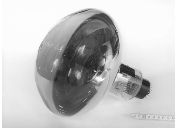
Figure 6.4: Left: Schematic view of an ANTARES optical module (OM). Right: A Hamamatsu R7081-20 10'' photomultiplier tube. Figures reproduced from Amram et al. (2002).
