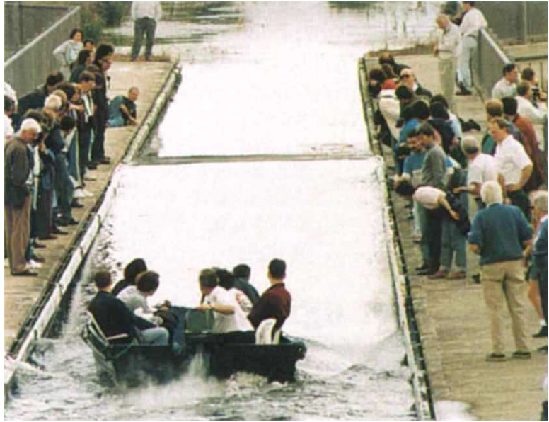
Figure 6: Modern-day reenactment of Scott Russell's discovery of solitons in the Union Canal. (Figure reprinted from "Soliton wave receives crowd of admirers" (1995), with license.) The soliton is visible as the "mountain" of water behind the boat.
