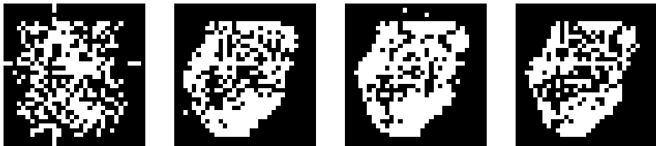
(b) Algorithm 7.1 with \tau = \frac{1}{32} . Number of projection angles: left: 2; mid-left: 6; mid-right: 10; right: 14.
