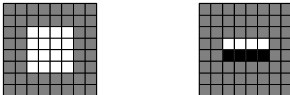
Figure 8.2: Two probe images. The pixels are colored as follows: black (0), grey (?), white (1). Left: homogeneous white region; right: horizontal edge at the bottom of a white region.
