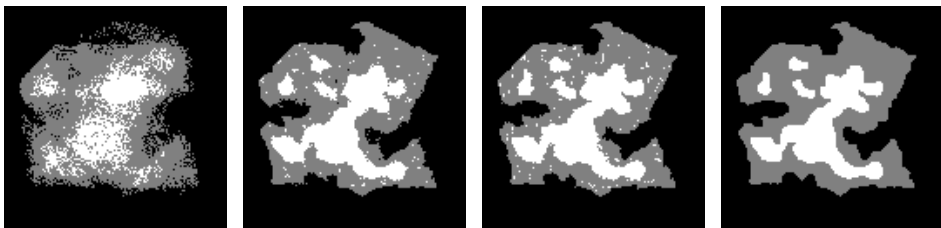
(d) Phantom 7.5(c). Alg. 7.1 with \tau = \frac{1}{\sqrt{128}} . N. proj. angles: left: 4; mid-left: 16; mid-right: 20; right: 24.
