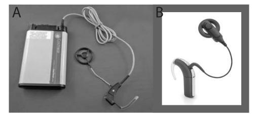
**Figure 4.** (A) Wearable Speech Processor (1982); measuring 11.7 cm x 7.6 cm x 2.1 cm and weighing 255 gram with batteries; (B) CP810 (2012); measuring 5.1 cm x 0.9 cm x 1.9 mm and weighing 10.9 gram. Both are Nucleus<sup>®</sup> speech processors from Cochlear<sup>TM</sup>, where (A) is the first processor, body worn and (B) is the most recent processor, worn behind the ear.
