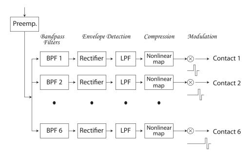
**Figure 6.** Block diagram of the Continues Interleaved Sampling (CIS) strategy. The signal is first pre-emphasized and filtered into six frequency bands. The envelopes of the filtered waveforms are then extracted by full-wave rectification and low-pass filtering. The envelope outputs are compressed to fit the patient's dynamic range and then modulated with biphasic pulses. The biphasic pulses are transmitted to the electrodes in an interleaved fashion.
