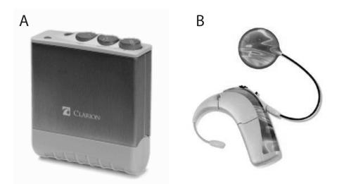
**Figure 7.** (A) Clarion CI device (1996); (B) Harmony processor (2010). Both are processors from Advanced Bionics<sup>®</sup>, where (A) is their first processor, body worn and (B) is the most recent processor, worn behind the ear.
