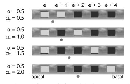
**Figure 2.** Explanation of the corrected  $\alpha$  ( $\alpha_c$ ), as defined by Equation 1. The light gray squares are the electrode contacts stimulated with current steering in the pitch discrimination experiment. The dots indicate the location associated with  $\alpha = 0.5$ , the actual fractions of the current going to the basal contact of the spanned pair.  $\alpha_c$  is after computing with Equation 1, expressed in electrode spacing.
