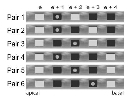
*Figure 3.* Electrode pairs used in pitch matching experiments. The light grey squares are the stimulated electrodes with dual-electrode stimulation. The dots correspond to the intermediate electrode contact i.e., the physical reference contact.
