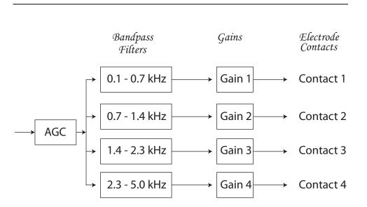
**Figure 5.** Block diagram of the compressed analog (CA) approach used in the Ineraid device. The signal is first compressed using an automatic gain control. The compressed signal is then filtered into four frequency bands (with the indicated frequencies), amplified using adjustable gain controls, and then sent directly to four intra cochlear electrodes.
