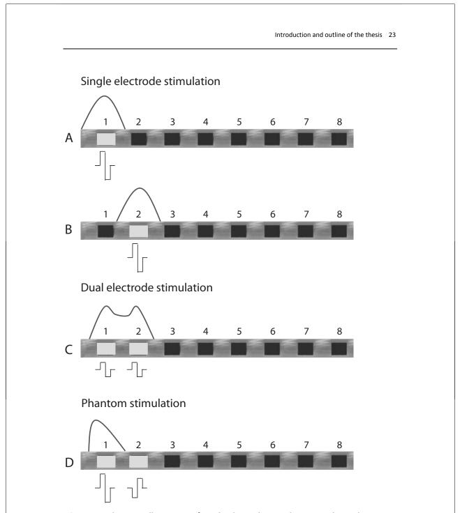
**Figure 9.** Schematic illustration of single electrode stimulation on electrode contact 1 (A) and contact 2 (B), dual electrode stimulation (C) and phantom stimulation (D). The light gray electrode contacts are the stimulated contacts. The curve in each panel is hypothetical sketch of the place neural response. Condition is indicated by pulse waveform(s) beneath the stimulated contacts on the electrode array.
