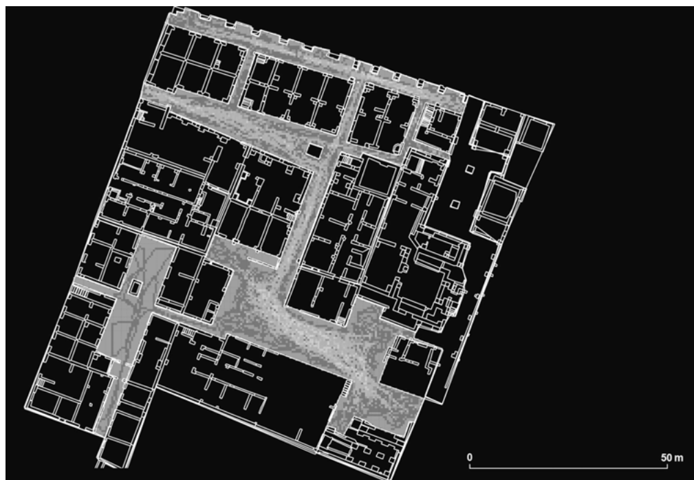
Figure 9 | Agent analysis (preliminary state) movement traces of 50 autonomous agents concentrated in the southern courtyard.
