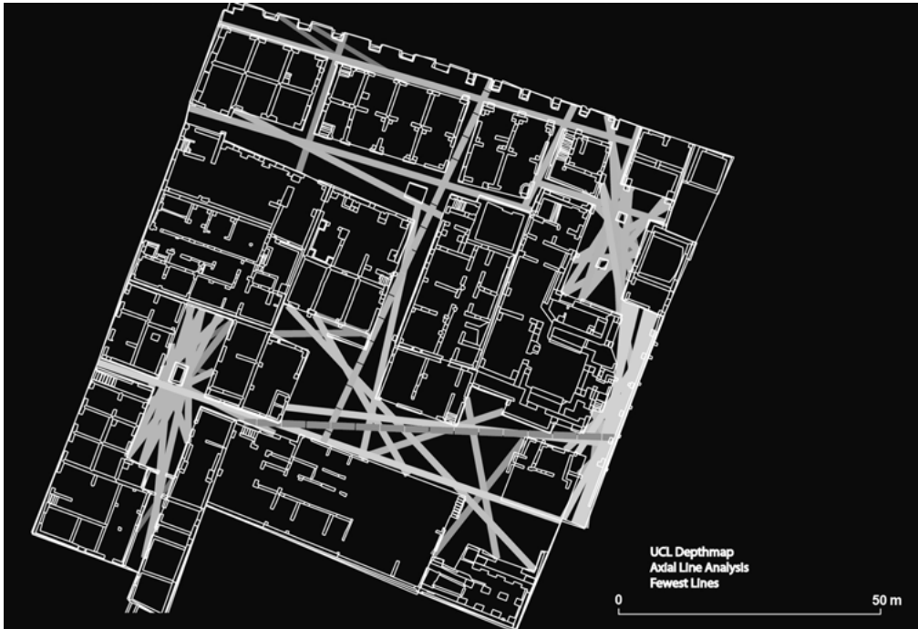
Figure 7 | The Insula's potential route matrix based on the longest and fewest lines; represented in greyscales. The movement spaces of the Terme del Faro are included in the analysis (Depthmap 7.12.00d; The Bartlett, University College London).
