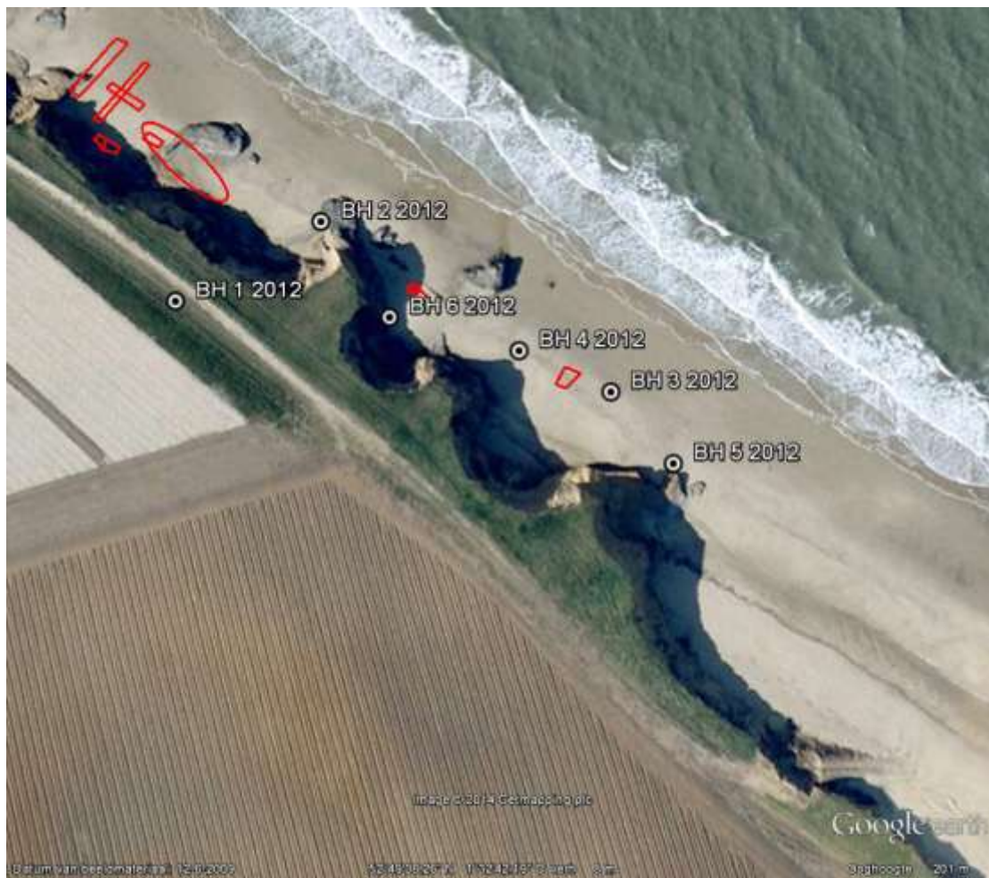
Figure 17 - Position of the 2012 boreholes relative to the excavation pits.
