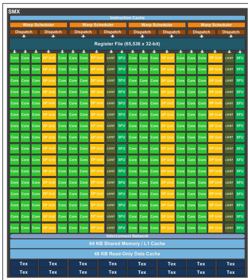
Figure 1.6: Kepler SMX: 192 single precision CUDA cores, 64 double precision units, 32 special function units (SFU), and 32 load/store units (LD/ST). Figure taken from (NVIDIA (2013b))
