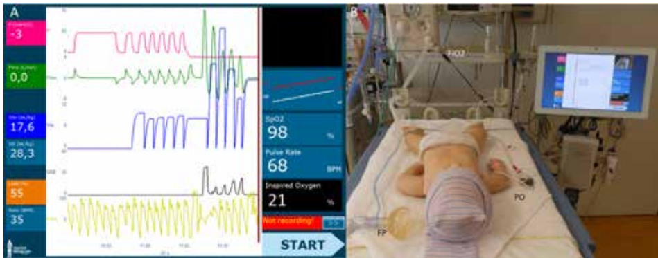
Figure 1. A) illustrates a respiratory tracing showing pressure (red), flow (green), expiratory volume (blue), capnography (black), HR plethysmography (black) in waveforms. Also it provides HR, oxygen saturation ( \text{SaO}_2 ), \text{FiO}_2 , inspiratory volume ( V_{ti} ), expiratory volume ( V_{te} ) and leak numerically. B) Shows a respiratory function monitor (Applied Biosignals, Weener, Germany) and set-up as currently used for physiological research of the newborn infant. The flow probe (FP) is connected to the face mask. Also an oxygen analyzer ( \text{FiO}_2 ) and Pulse oximeter can be added to monitor supplied oxygen as well as oxygen saturation and heart rate.
