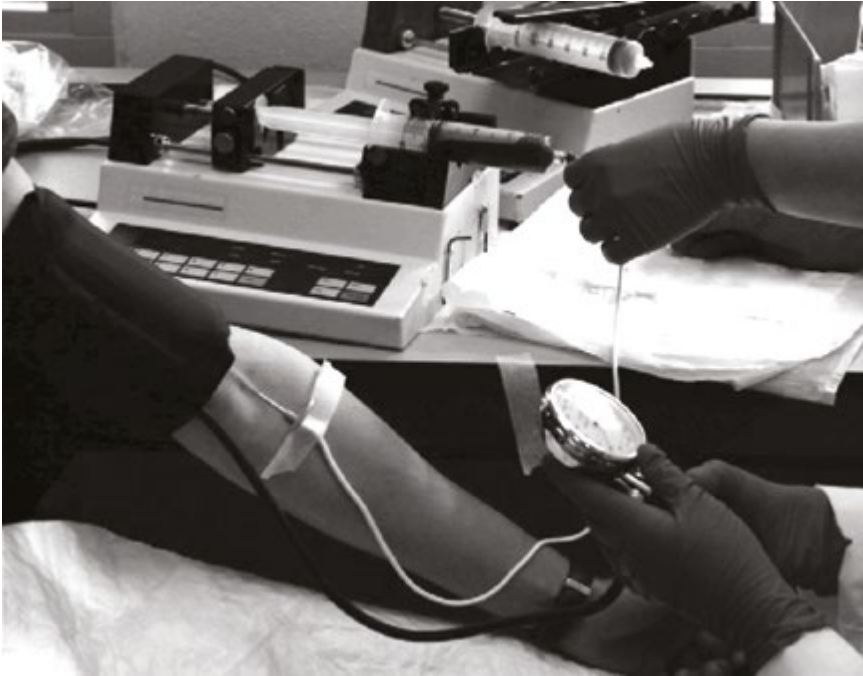
Figure 2. Ex vivo perfusion model using a cuff at a constant pressure of 45 mmHg to ensure blood flow. Blood is aspirated through the graft with a constant flow of 20 mL/min, resulting in a shear rate of 74/s.
