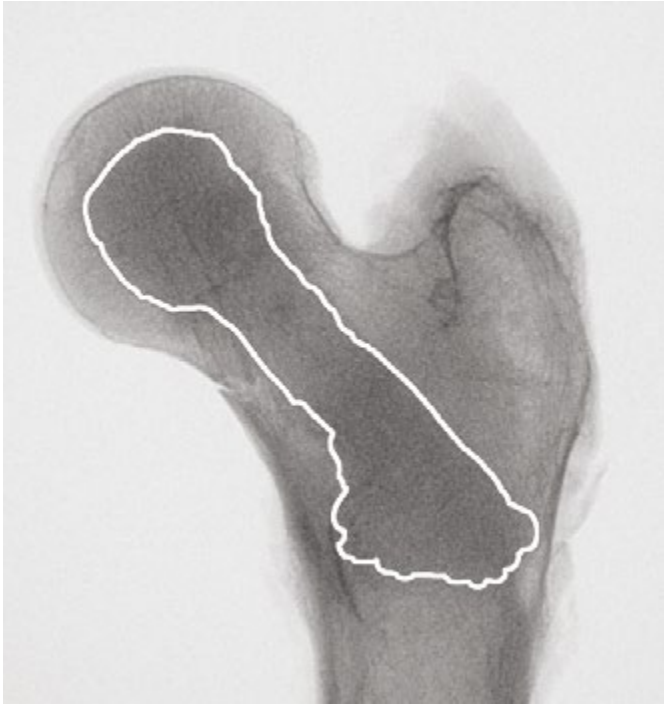
Figure 2. X-ray image of a Silicone augmented proximal femur. The line marks the deposition of the Silicone.
