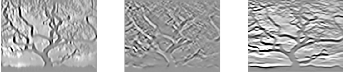
Figure A7. From left to right: H_{xx} , H_{xy} and H_{yy} for \sigma = 6 pixels. Notice that H_{xx} and H_{yy} enhance the vertical and horizontal ridges, respectively, while the H_{xy} enhances the diagonal ridges.
