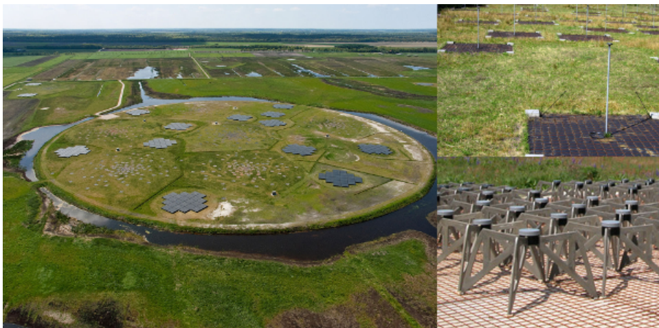
Figure 1.3: The LOFAR superterp near Exloo, Netherlands, showing several stations with both HBA and LBA antennae (left). Individual LBA (top right) and HBA (bottom right). (credit LOFAR/ASTRON).
