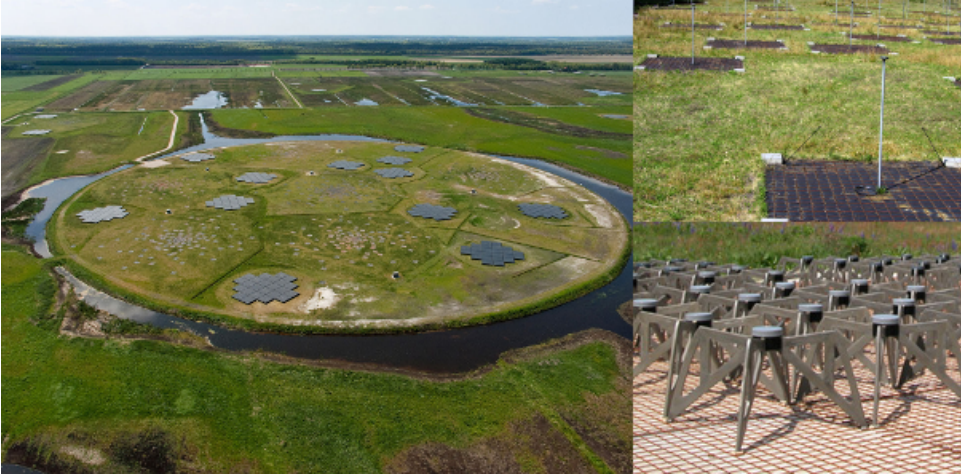
Figure 2: The LOFAR superterp near Exloo, Netherlands, showing several stations with both HBA and LBA antennae ( left ). Individual LBA ( top right ) and HBA ( bottom right ). (credit LOFAR/ASTRON).
