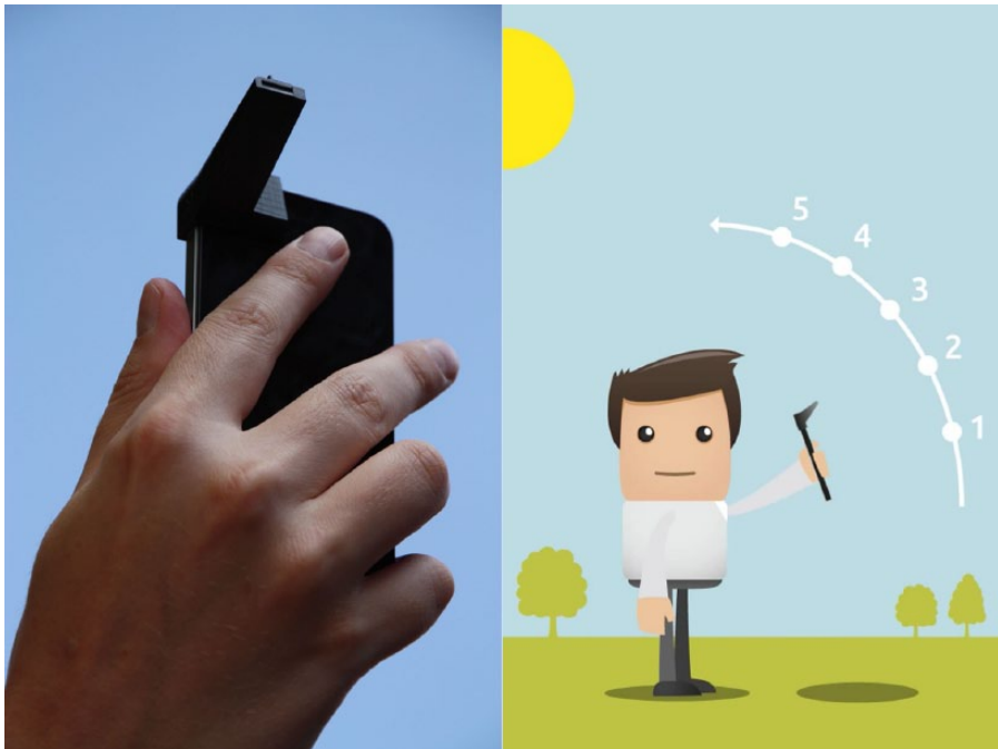
Figure 1. The iSPEX add-on on a smartphone on the left, instruction for taking measurements on the right.
