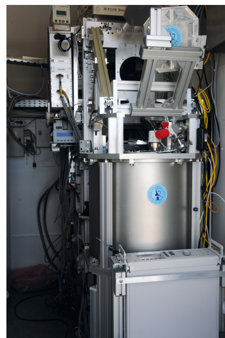
Figure 1. The SEPIA instrument installed at APEX.
