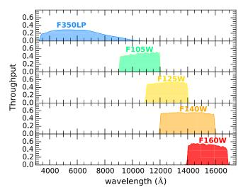
**Figure 1.** Transmission curves of our filter set, from visible to IR: F350LP, F105W ( $Y_{105}$ ), F125W ( $J_{125}$ ), F140W ( $JH_{140}$ ), and F160W ( $H_{160}$ ) as labeled. We used two complementary, non-overlapping sets of IR filters, namely  $Y_{105}$ – $JH_{140}$  and  $J_{125}$ – $H_{160}$ , for an optimal identification of high-z galaxies through the dropout technique (Stanway et al. 2008).
