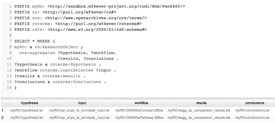
Figure 10 Screenshot showing a SPARQL query and its results. Query to obtain a reference to the data that was used as input to our workflows and the conclusions that we drew from evaluating the workflow results.
