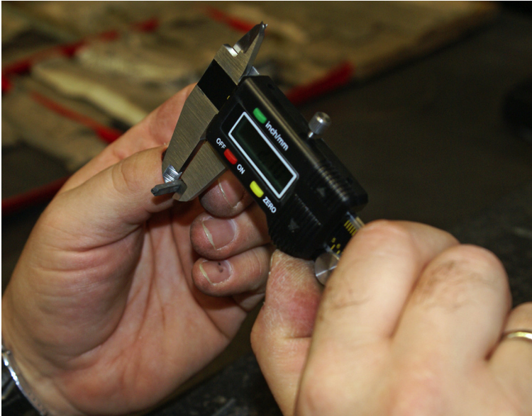
Figure A5.12 Digital calliper with Renaissance foundry type.
