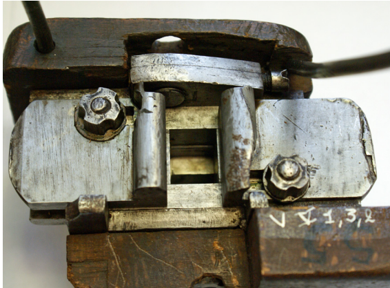
Figure 6.4 The aperture in the centre is the result of sliding the two halves.
