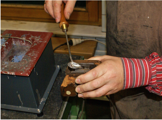
Figure 6.6 Molten lead is poured into the shank.
