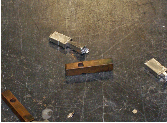
Figure 6.8 The tang is a wedge-shaped tail.
