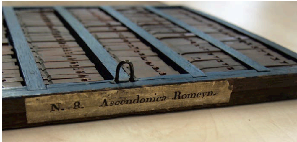
Figure 9.3 The MA8 set containing the Ascendonica Romain matrices justified by Van den Keere.
