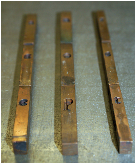
Figure 7.9 Matrices of the Gros Canon Romain showing groups of equal widths.
