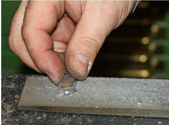
Figure 6.9 The rough edges are filed.
