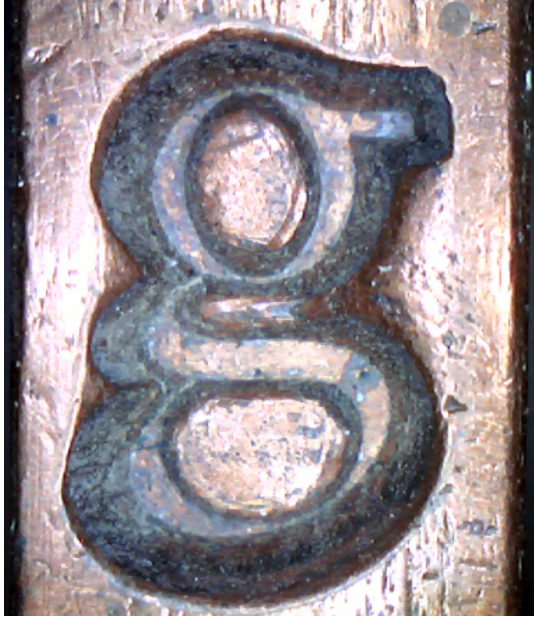
Figure 7.11 Digital microscope photo of the Moyen Canon Romain matrix for the lowercase g.
