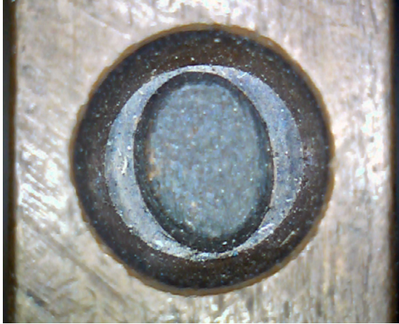
Figure 7.8 Digital-microscope photo of the Gros Canon Romain matrix for the lowercase o.
