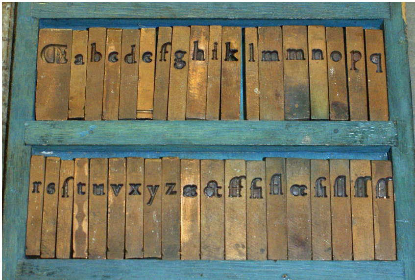
Figure 7.6 Matrices of Garamont's Gros Canon Romain.
