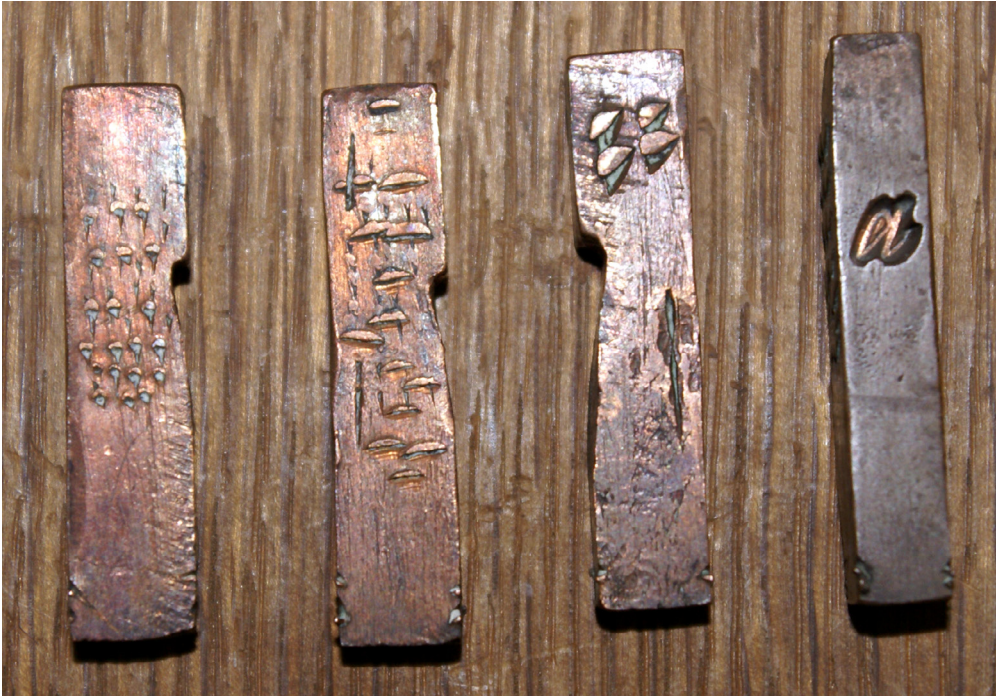
Figure A5.7 Excrescences on the sides of the matrices of the Ascendonica Cursive.
