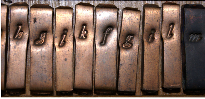
Figure A5.2 Unjustified matrices of Granjon's Ascendonica Cursive.
