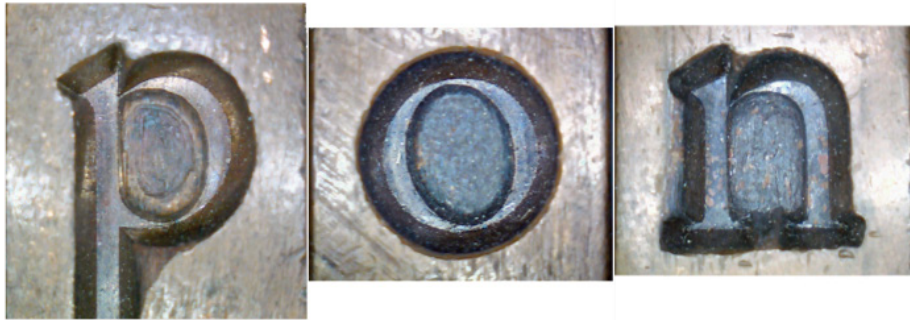
Figure 7.10 Word typeset in Gros Canon Romain matrices.
