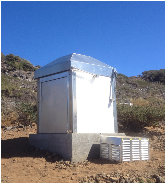
Fig. 1. Northern MASCARA station on La Palma (Spain). The box next to the station contains the heat exchanger used in the decommissioned liquid cooling system.
