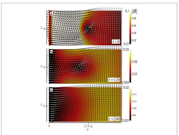
**Figure 4.** Cut through the x–z plane showing the disappearance of the circular null line. (a) Initial field, (b) field at time t = 120, and (c) disappearance of the null line by merging with the straight null on the z-axis at t = 240.
