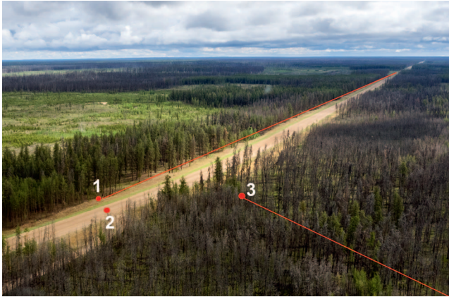
FIGURE 1. Sampling design schematic for our experiments near Calling Lake, Alberta, Canada, July 22–August 24, 2014. Wildlife Acoustics SM2 recorders were placed on the forest edge (1) and on the road (2), and playbacks were conducted to both recorders simultaneously along a transect following the forest edge. For forest playbacks, recorders were placed within the interior forest (3) and playback transects ran perpendicular to the road.
