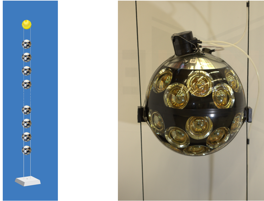
Figure 18: A drawing of KM 3 Net detection units and a photo of a KM 3 Net module attached to a string.
