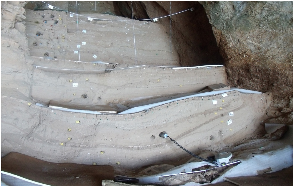
Fig. 1.6.13 In situ gamma spectrometry measurement using a \text{LaBr}_3 detector at an OSL sample hole at Vanguard Cave, Gibraltar.
