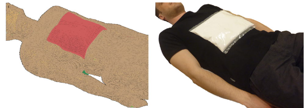
FIGURE 1. (left) Schematic of the setup for the EM simulations with a dielectric pad (red) with thickness 1 cm placed on the abdomen. An identically shaped pad (green) is placed on the back, in the same position. (right) photo-
