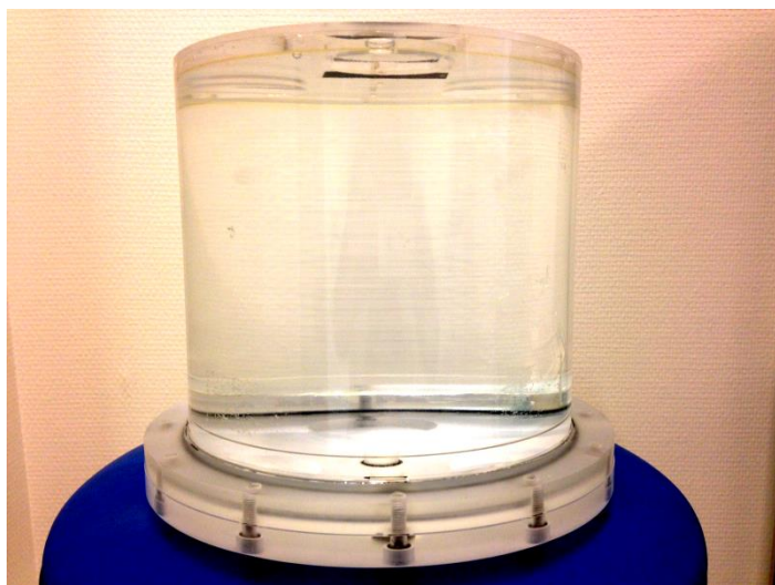
Figure 1. Cylindrical water tank phantom. Diameter: 20 cm; length: 25 cm.
