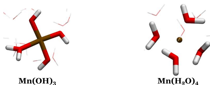
Figure A4.1 The different solvation environments observed around the Mn ion when the environment is not constrained.
