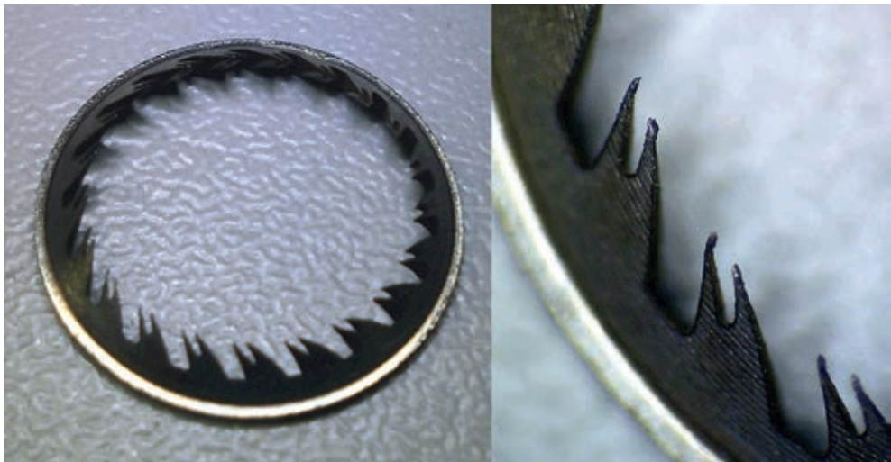
Figure 7: Prototyped steel teeth ring, using tooth geometry J (Fig. 10, bottom), 2.0 mm height, 1.4 mm width, 0.3 mm spacing between teeth, and 45° inward angle. The ring has 21 teeth.
