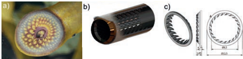
Figure 3: (a) Lamprey. Image edited to only show the mouth [93]. (b) Lamprey inspired morcellation instrument tip, having integrated teeth for tissue traction. (c) Design of a single teeth ring. Dimensions are in millimetres.
