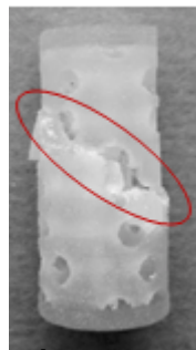
Fig. 4. The specimen after compression test
