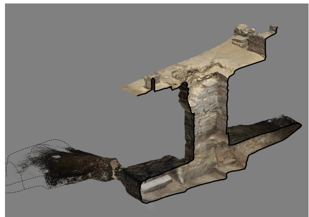
Fig. 19: Longitudinal section of shaft 131 and underground chambers seen from the south-west. The image also shows the small breach in the north-west corner of room A, connecting this room to other underground chambers, which are sketched with a dashed line. Image by 3D Survey Group, Politecnico di Milano/Leiden-Turin Expedition to Saqqara.
