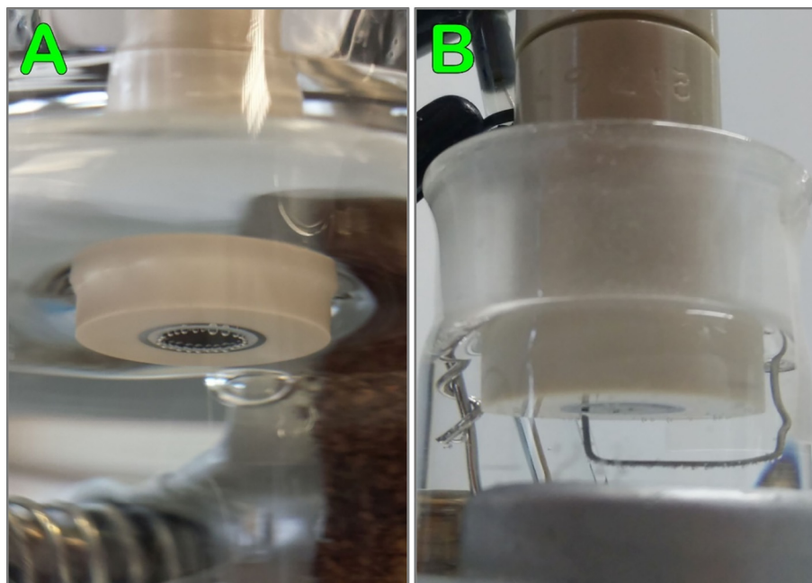
Fig. 2. Photographs of a rotating electrode equipped with an IrO x /GC disk (black) and Pt ring (grey). A: Tip after an experiment involving vigorous gas evolution, during which the collection factor became severely distorted. B: Tip during attempts to dislodge gas bubbles using a Ti wire. The Ti wire is mounted under the tip, with its point aimed at the disk-Teflon spacer boundary. Accumulating bubbles collided with the wire and were 'pushed off' during rotation.
