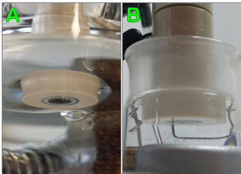
Figure 8.2: Photographs of a rotating electrode equipped with an \text{IrO}_x/\text{GC} disk (black) and Pt ring (grey). A: Tip after an experiment involving vigorous gas evolution, during which the collection factor became severely distorted. B: Tip during attempts to dislodge gas bubbles using a Ti wire. The Ti wire is mounted under the tip, with its point aimed at the disk-Teflon spacer boundary. Accumulating bubbles collided with the wire and were 'pushed off' during rotation.
