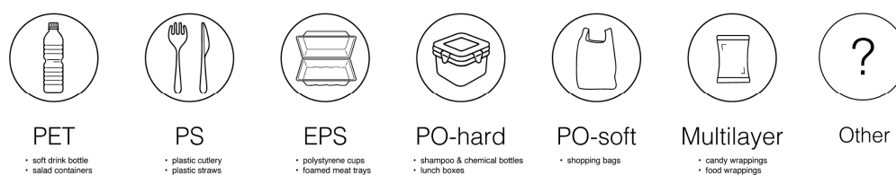
Figure 3. The categories used for classification in this research, including some typical items that belong to these classes. Items that cannot be identified as one of the six specific classes are categorized as “other”.
