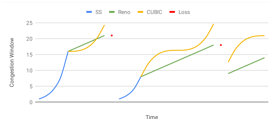
Fig. 2.2 Schematic behavior comparison of Reno and CUBIC loss-based congestion controls.
