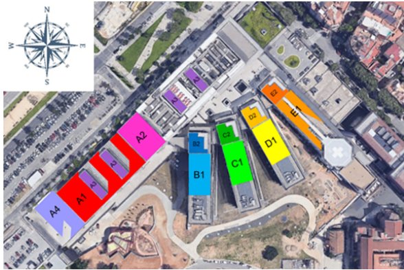
Figure 4. Available roof areas of the hospital.
