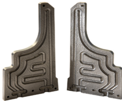
Figure 10. AM tool and die with conformal cooling channels [111].
