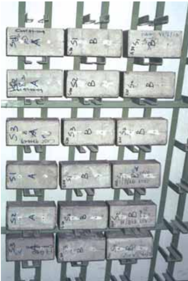
Figure 2: Companion drying shrinkage samples
