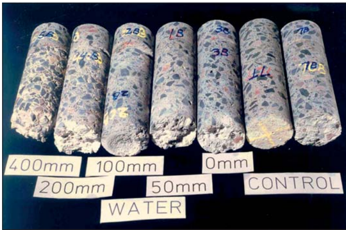
Figure 2 Concrete cores from concrete cast into water in “pile holes”
