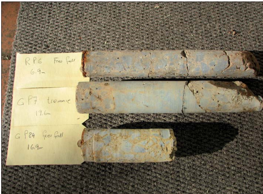
Figure 10 Relative comparison of free-fall and tremie-placed concrete
