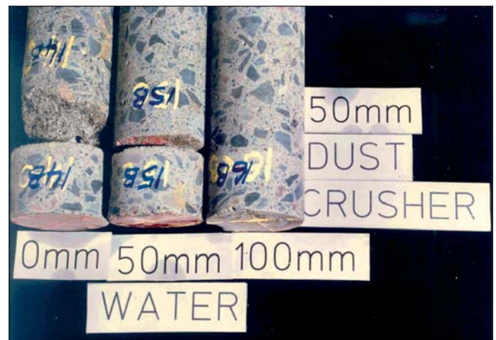
Figure 8 Close-up of contact between “pile” concrete and blinding concrete for “piles” cast with a 50 mm layer of crusher dust at the bottom of the “pile hole”
