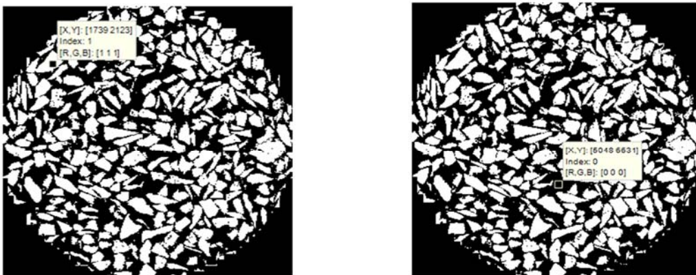
Figure 4. Binary image for easier calculation of the total number of particles across the image
