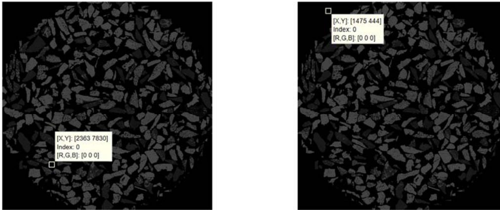
Figure 3. Background conversion of the background within to make it the same as the background from outside the polished section frame.
