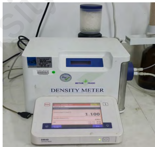
Figure 3.21: DE-40 density meter, Mettler Toledo
