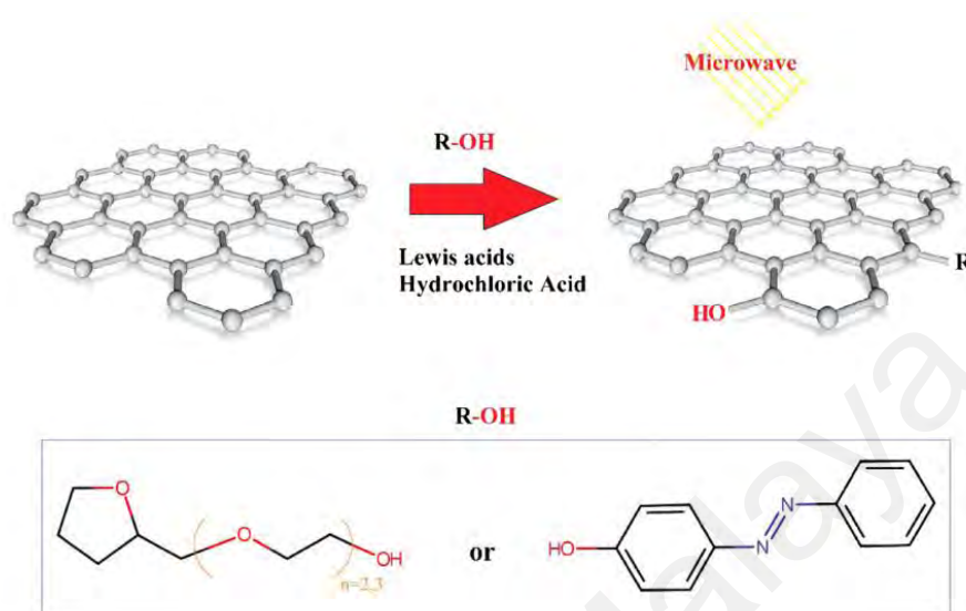
Figure 2.12: Experimental procedure for chemical-assisted functionalization of GNP with PEG and Azo (Amiri, Shanbedi, et al., 2015)
