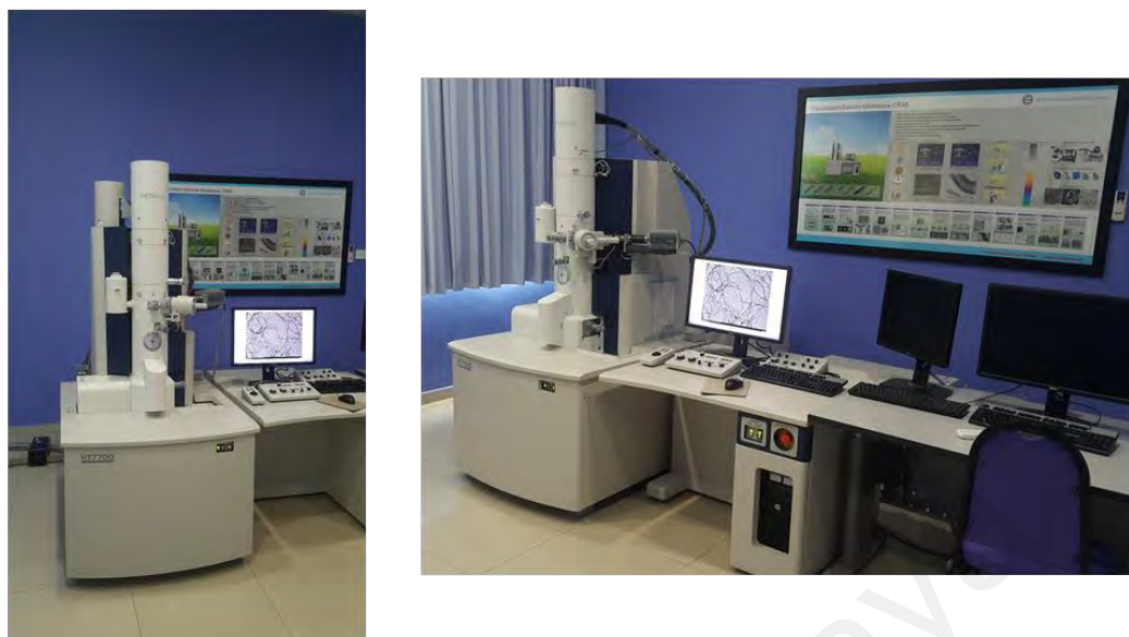
Figure 3.16: Hitachi HT7700 transmission electron microscope
