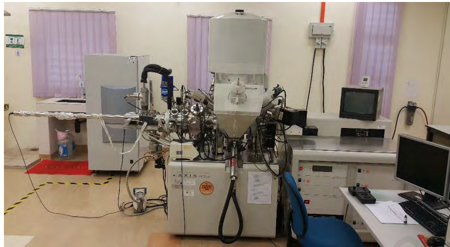
Figure 3.15: Axis Ultra-DLD system, Kratos Analytical X-ray photoemission spectrometer (XPS)
